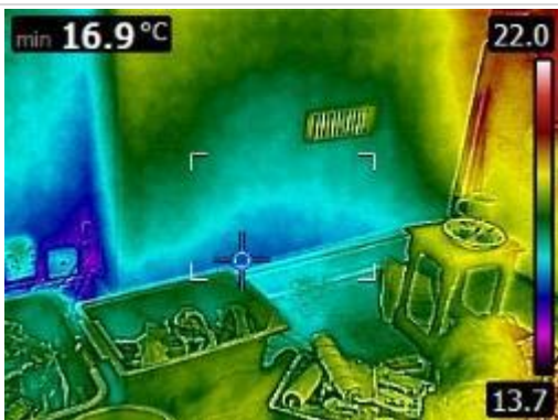
Thermal image of fireplace in lounge/diner showing areas of elevated moisture readings. Blue is area of elevated readings.
