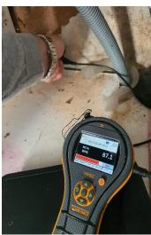
As you can see from the above photos at the time of our visit, we have recorded elevated to very high moisture readings on the lower external wall, floor, base cupboard side panel (which is water stained), and back of the sink cupboard.
