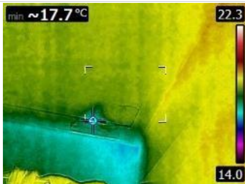
Thermal image of water damaged area of bedroom ceiling, coving and upper wall.
